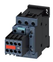
power contactor, AC-3e/AC-3, 32 A, 15 kW / 400 V, 3-pole, 110 V AC, 50 Hz / 120 V, 60 Hz, with plugged-in varistor, auxiliary contacts: 2 NO + 2 NC, screw terminal, size: S0, captive auxiliary switch
