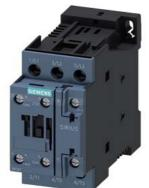
power contactor, AC-3e/AC-3, 32 A, 15 kW / 400 V, 3-pole, 21-28 V AC/DC, 50/60 Hz, with integrated varistor, auxiliary contacts: 1 NO + 1 NC, screw terminal, size: S0
