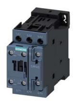
power contactor, AC-3e/AC-3, 32 A, 15 kW / 400 V, 3-pole, 95-130 V AC/DC, 50/60 Hz, with integrated varistor, auxiliary contacts: 1 NO + 1 NC, screw terminal, size: S0
