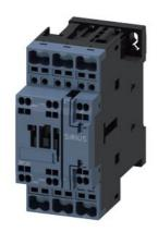
power contactor, AC-3e/AC-3, 32 A, 15 kW / 400 V, 3-pole, 42 V AC, 50/60 Hz, auxiliary contacts: 1 NO + 1 NC, spring-loaded terminal, size: S0, upright mounting position
