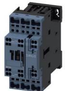
power contactor, AC-3e/AC-3, 32 A, 15 kW / 400 V, 3-pole, 48 V AC, 50 Hz, auxiliary contacts: 1 NO + 1 NC, spring-loaded terminal, size: S0
