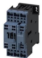
power contactor, AC-3e/AC-3, 32 A, 15 kW / 400 V, 3-pole, 110 V AC, 50 Hz / 120 V, 60 Hz, auxiliary contacts: 1 NO + 1 NC, spring-loaded terminal, size: S0, upright mounting position
