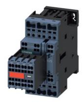
power contactor, AC-3e/AC-3, 32 A, 15 kW / 400 V, 3-pole, 230 V AC, 50/60 Hz, auxiliary contacts: 2 NO + 2 NC, spring-loaded terminal, size: S0, captive auxiliary switch, no surge suppressor retrofittable
