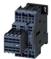
power contactor, AC-3e/AC-3, 32 A, 15 kW / 400 V, 3-pole, 230 V AC, 50 Hz, auxiliary contacts: 2 NO + 2 NC, spring-loaded terminal, size: S0, removable auxiliary switch
