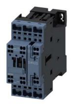
power contactor, AC-3e/AC-3, 32 A, 15 kW / 400 V, 3-pole, 24 V DC, auxiliary contacts: 1 NO + 1 NC, spring-loaded terminal, size: S0, communication-capable
