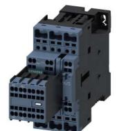
power contactor, AC-3e/AC-3, 32 A, 15 kW / 400 V, 3-pole, 24 V DC, auxiliary contacts: 2 NO + 2 NC, spring-loaded terminal, size: S0, removable auxiliary switch
