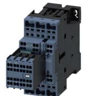
power contactor, AC-3e/AC-3, 32 A, 15 kW / 400 V, 3-pole, 110 V DC, auxiliary contacts: 2 NO + 2 NC, spring-loaded terminal, size: S0, removable auxiliary switch
