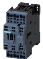
power contactor, AC-3e/AC-3, 32 A, 15 kW / 400 V, 3-pole, 48 V DC, auxiliary contacts: 1 NO + 1 NC, spring-loaded terminal, size: S0
