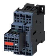
power contactor, AC-3e/AC-3, 32 A, 15 kW / 400 V, 3-pole, 24 V DC, with plugged-in varistor, auxiliary contacts: 2 NO + 2 NC, spring-loaded terminal, size: S0, captive auxiliary switch
