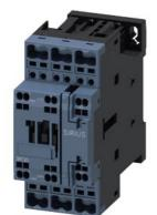
power contactor, AC-3e/AC-3, 32 A, 15 kW / 400 V, 3-pole, 230 V AC, 50 Hz, with plugged-in RC element, auxiliary contacts: 1 NO + 1 NC, spring-loaded terminal, size: S0
