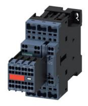
power contactor, AC-3e/AC-3, 32 A, 15 kW / 400 V, 3-pole, 24 V DC, with plugged-in diode combination, auxiliary contacts: 2 NO + 2 NC, spring-loaded terminal, size: S0, captive auxiliary switch
