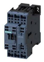
power contactor, AC-3e/AC-3, 32 A, 15 kW / 400 V, 3-pole, 12 V DC, 0.7-1.25\* Us, with plugged-in varistor, auxiliary contacts: 1 NO + 1 NC, spring-loaded terminal, size: S0, suitable for PLC outputs, not expandable with auxiliary switch
