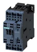
power contactor, AC-3e/AC-3, 32 A, 15 kW / 400 V, 3-pole, 24 V DC, 0.7-1.25\* Us, with plugged-in varistor, auxiliary contacts: 1 NO + 1 NC, spring-loaded terminal, size: S0, suitable for PLC outputs, not expandable with auxiliary switch
