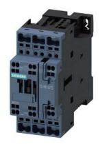
power contactor, AC-3e/AC-3, 32 A, 15 kW / 400 V, 3-pole, 125 V DC, 0.7-1.25  $^{\star}$  Us, with plugged-in varistor, auxiliary contacts: 1 NO + 1 NC, spring-loaded terminal, size: S0, suitable for PLC outputs, not expandable with auxiliary switch
