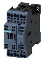
power contactor, AC-3e/AC-3, 32 A, 15 kW / 400 V, 3-pole, 21-28 V AC/DC, 50/60 Hz, with integrated varistor, auxiliary contacts: 1 NO + 1 NC, spring-loaded terminal, size: S0
