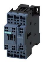
power contactor, AC-3e/AC-3, 32 A, 15 kW / 400 V, 3-pole, 95-130 V AC/DC, 50/60 Hz, with integrated varistor, auxiliary contacts: 1 NO + 1 NC, spring-loaded terminal, size: S0
