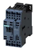
power contactor, AC-3e/AC-3, 32 A, 15 kW / 400 V, 3-pole, 200-280 V AC/DC, 50/60 Hz, with integrated varistor, auxiliary contacts: 1 NO + 1 NC, spring-loaded terminal, size: S0
