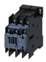
power contactor, AC-3e/AC-3, 32 A, 15 kW / 400 V, 3-pole, 24 V DC, auxiliary contacts: 1 NO + 1 NC, ring cable lug connection, size: S0  $\,$
