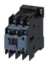
power contactor, AC-3e/AC-3, 32 A, 15 kW / 400 V, 3-pole, 24 V DC, 0.7-1.25\* Us, with plugged-in varistor, auxiliary contacts: 1 NO + 1 NC, ring cable lug connection, size: S0, suitable for PLC outputs, not expandable with auxiliary switch
