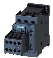
power contactor, AC-3e/AC-3, 38 A, 18.5 kW / 400 V, 3-pole, 24 V AC, 50/60 Hz, auxiliary contacts: 2 NO + 2 NC, screw terminal, size: S0, removable auxiliary switch
