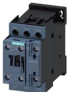
power contactor, AC-3e/AC-3, 38 A, 18.5 kW / 400 V, 3-pole, 42 V AC, 50/60 Hz, auxiliary contacts: 1 NO + 1 NC, screw terminal, size: S0, India 40 A, Tu max. 50  $^\circ\text{C}$
