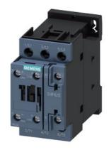
power contactor, AC-3e/AC-3, 38 A, 18.5 kW / 400 V, 3-pole, 110 V AC, 50/60 Hz, auxiliary contacts: 1 NO + 1 NC, screw terminal, size: S0
