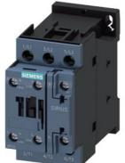
power contactor, AC-3e/AC-3, 38 A, 18.5 kW / 400 V, 3-pole, 48 V AC, 50/60 Hz, auxiliary contacts: 1 NO + 1 NC, screw terminal, size: S0
