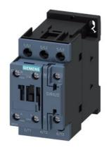
power contactor, AC-3e/AC-3, 38 A, 18.5 kW / 400 V, 3-pole, 110 V AC, 50 Hz / 120 V, 60 Hz, auxiliary contacts: 1 NO + 1 NC, screw terminal, size: S0, multi-unit packaging, pack = 24 units
