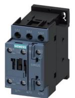
power contactor, AC-3e/AC-3, 38 A, 18.5 kW / 400 V, 3-pole, 230 V AC, 50/60 Hz, auxiliary contacts: 1 NO + 1 NC, screw terminal, size: S0, reusable packaging, pack = 48 units
