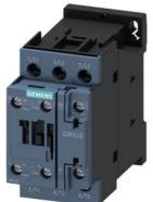
power contactor, AC-3e/AC-3, 38 A, 18.5 kW / 400 V, 3-pole, 230 V AC, 50/60 Hz, auxiliary contacts: 1 NO + 1 NC, screw terminal, size: S0
