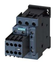
power contactor, AC-3e/AC-3, 38 A, 18.5 kW / 400 V, 3-pole, 220 V AC, 50/60 Hz, auxiliary contacts: 2 NO + 2 NC, screw terminal, size: S0, removable auxiliary switch
