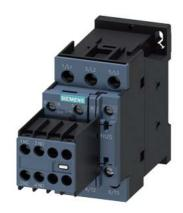
power contactor, AC-3e/AC-3, 38 A, 18.5 kW / 400 V, 3-pole, 230 V AC, 50 Hz, auxiliary contacts: 2 NO + 2 NC, screw terminal, size: S0, removable auxiliary switch, reusable packaging, pack = 48 units
