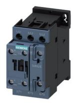
power contactor, AC-3e/AC-3, 38 A, 18.5 kW / 400 V, 3-pole, 380 V AC, 50/60 Hz, auxiliary contacts: 1 NO + 1 NC, screw terminal, size: S0
