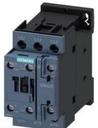
power contactor, AC-3e/AC-3, 38 A, 18.5 kW / 400 V, 3-pole, 400 V AC, 50 Hz, auxiliary contacts: 1 NO + 1 NC, screw terminal, size: S0, India 40 A, Tu max. 50  $^\circ\text{C}$
