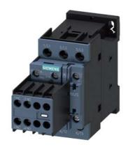
power contactor, AC-3e/AC-3, 38 A, 18.5 kW / 400 V, 3-pole, 400 V AC, 50 Hz, auxiliary contacts: 2 NO + 2 NC, screw terminal, size: S0, removable auxiliary switch
