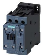
power contactor, AC-3e/AC-3, 38 A, 18.5 kW / 400 V, 3-pole, 24 V DC, auxiliary contacts: 1 NO + 1 NC, screw terminal, size: S0, communication-capable
