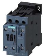
power contactor, AC-3e/AC-3, 38 A, 18.5 kW / 400 V, 3-pole, 24 V DC, auxiliary contacts: 1 NO + 1 NC, screw terminal, size: S0
