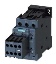
power contactor, AC-3e/AC-3, 38 A, 18.5 kW / 400 V, 3-pole, 24 V DC, auxiliary contacts: 2 NO + 2 NC, screw terminal, size: S0, removable auxiliary switch, reusable packaging, pack = 48 units
