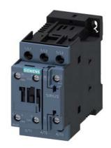
power contactor, AC-3e/AC-3, 38 A, 18.5 kW / 400 V, 3-pole, 110 V DC, auxiliary contacts: 1 NO + 1 NC, screw terminal, size: S0, India 40 A, Tu max. 50  $^{\circ}$ C
