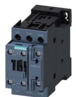
power contactor, AC-3e/AC-3, 38 A, 18.5 kW / 400 V, 3-pole, 220 V DC, auxiliary contacts: 1 NO + 1 NC, screw terminal, size: S0, India 40 A, Tu max. 50  $^\circ\text{C}$
