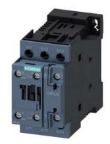
power contactor, AC-3e/AC-3, 38 A, 18.5 kW / 400 V, 3-pole, 220 V DC, auxiliary contacts: 1 NO + 1 NC, screw terminal, size: S0  $\,$
