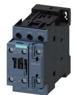
power contactor, AC-3e/AC-3, 38 A, 18.5 kW / 400 V, 3-pole, 24 V DC, with plugged-in diode combination, auxiliary contacts: 1 NO + 1 NC, screw terminal, size: S0
