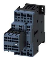
power contactor, AC-3e/AC-3, 38 A, 18.5 kW / 400 V, 3-pole, 24 V AC, 50 Hz, auxiliary contacts: 2 NO + 2 NC, spring-loaded terminal, size: S0, removable auxiliary switch
