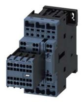
power contactor, AC-3e/AC-3, 38 A, 18.5 kW / 400 V, 3-pole, 24 V AC, 50/60 Hz, auxiliary contacts: 2 NO + 2 NC, spring-loaded terminal, size: S0, removable auxiliary switch
