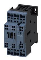
power contactor, AC-3e/AC-3, 38 A, 18.5 kW / 400 V, 3-pole, 230 V AC, 50/60 Hz, auxiliary contacts: 1 NO + 1 NC, spring-loaded terminal, size: S0, upright mounting position
