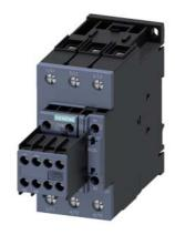
power contactor, AC-3e/AC-3, 65 A, 30 kW / 400 V, 3-pole, 110 V AC, 50/60 Hz, auxiliary contacts: 2 NO + 2 NC, screw terminal, size: S2, removable auxiliary switch
