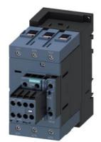
power contactor, AC-3e/AC-3, 80 A, 37 kW / 400 V, 3-pole, 24 V AC, 50/60 Hz, auxiliary contacts: 2 NO + 2 NC, screw terminal, size: S3, removable auxiliary switch
