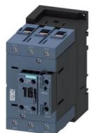
contactor, NEMA version, 50 HP, 460 / 575 V, 3-pole, 220 V AC, 50 Hz / 240 V, 60 Hz, auxiliary contacts: 1 NO + 1 NC, screw terminal, size: S3  $\,$
