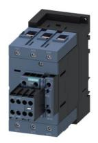
power contactor, AC-3e/AC-3, 95 A, 45 kW / 400 V, 3-pole, 220 V AC, 50 Hz / 240 V, 60 Hz, auxiliary contacts: 2 NO + 2 NC, screw terminal, size: S3, removable auxiliary switch
