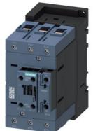
power contactor, AC-3e/AC-3, 95 A, 45 kW / 400 V, 3-pole, 415 V AC, 50 Hz, auxiliary contacts: 1 NO + 1 NC, screw terminal, size: S3  $\,$
